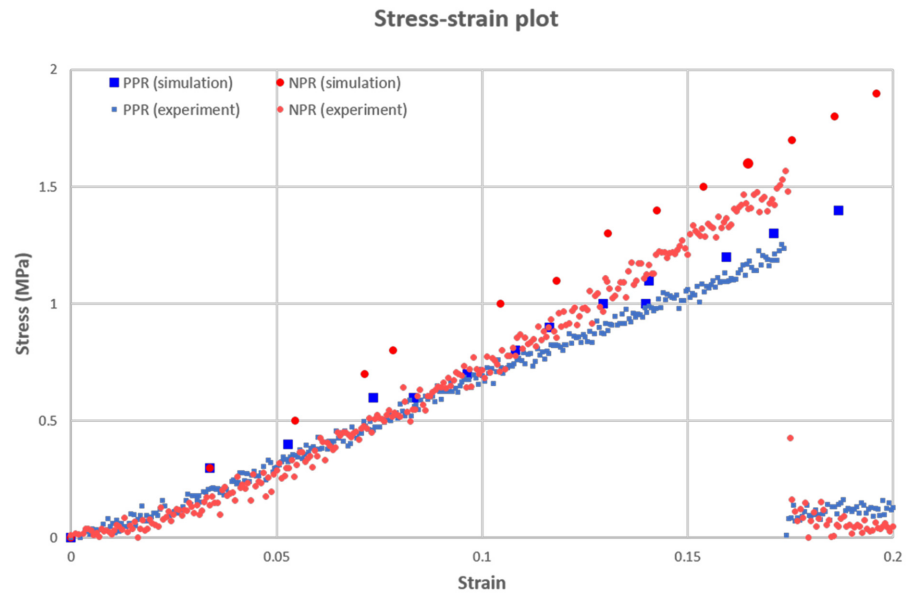
Fig 7. Stress-strain plot of the simulation and experiment at the PPR and NPR constructs. (Large blue-color square: simulation result at PPR construct, Large red-color circle: simulation result at NPR construct, small blue-color square: experiment result at PPR construct, small red-color circle: experiment result at NPR construct.)
