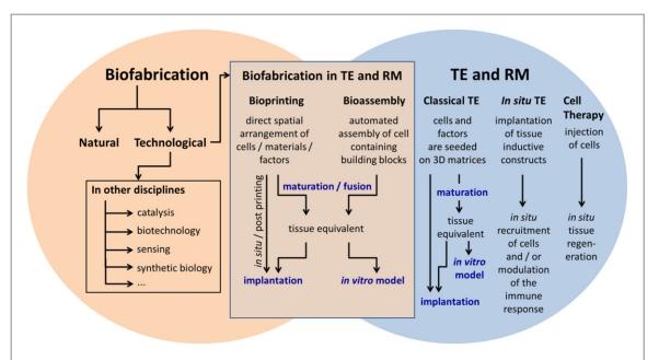
**Figure 2.** The term Biofabrication is used to describe natural processes such as biomineralization and technological processes in various disciplines such as catalysis, biotechnology, sensing, synthetic biology, and especially TE and RM. For application within TE and RM, Biofabrication can generally be divided into two distinct approaches, Bioprinting and Bioassembly.
